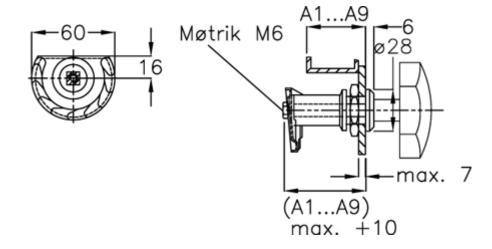
Door + frame thickness = 22-30Measure type = A2
